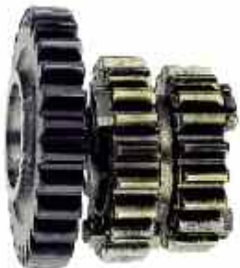
Gears from a motorcycle spur gear transmission after loss of oil: BALINIT® C (WC/C)-coated (left), uncoated (right)
