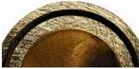
Bronze: abrasive wear and deformation
