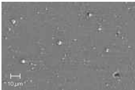
Surface of a PVD arc coating with droplets, without finishing
