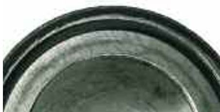
Steel and BALINIT® C (WC/C): wear < 1 µm
